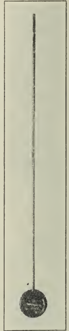
Fig. 4. Long-stemmed indicating thermometer suitable for taking the temperature of must in fermentation.
